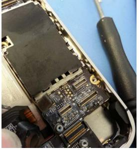
Water damage inside a cell phone causing corrosion. Via <u>Monterey Computer Repair</u>.
